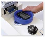
Novel bath design utilizes unique easy-locking base for secure and simple attachment; no risk of fluid leaking into the instrument.
